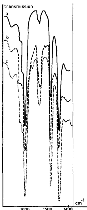
FIG. 7. Spectra of pyridine chemisorbed on CO-reduced \text{Cu}^{2+}\text{Y} : (a) pyridine evacuated at 150^\circ\text{C} , (b) exposed to water and re-evacuated at 150^\circ\text{C} , and (c) sample reduced by CO in the presence of small amount of water.
